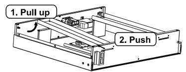
**Note:** To install the second branch of batteries, repeat the same procedures on the battery fixing plate on the right side of battery box.
