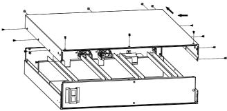
Step 5: Once battery box is opened, remove the battery fixing plate present on the left side of the battery box by unscrewing the 2 screws present.
