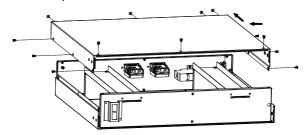
Step 5: Once the battery box is opened, remove the battery fixing plate present on the left side of the unit by unscrewing the 2 screws.
