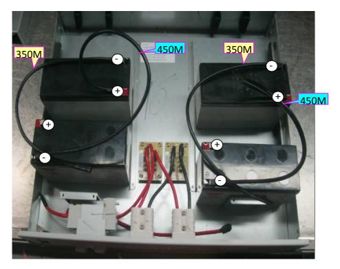
**Note:** The cable connection from external battery connector to PCB is already present inside the battery box. All the other cable connection should be followed by wiring diagram.
