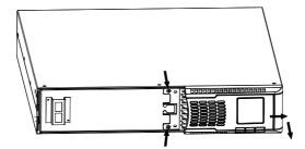
Step 4: Remove the metal top cover of the battery box by unscrewing 8 screws present on the two sides (4 on the right side and 4 on the left side), 3 screws on the top and 4 screws on the back side.
