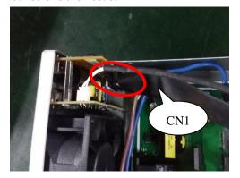
**Step 11:** Use 14-pin signal cable to connect CN11 of control board and CN1 point of parallel board.
