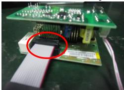
**Step 9:** Install and screw parallel board tightly like that. Four screws are needed.
