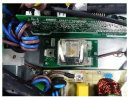
**Step 3:** Remove the screws of TB and COMMU board as shown in figure.
