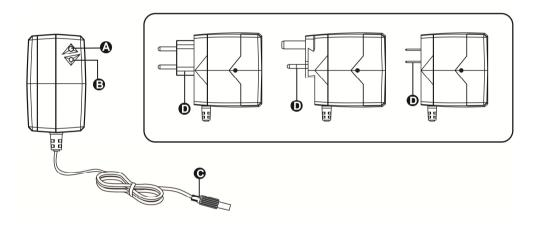
A Restart/Off Button B LED indicator C DC output connector D AC input
